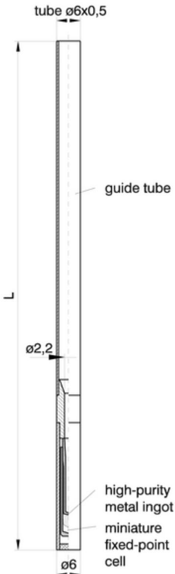
Stainless steel tube with firmly installed miniature fixed-point cell, used for an easy calibration of slender temperature sensors ( $< \varnothing 2 \text{ mm}$ ), or their whole measuring circuits
