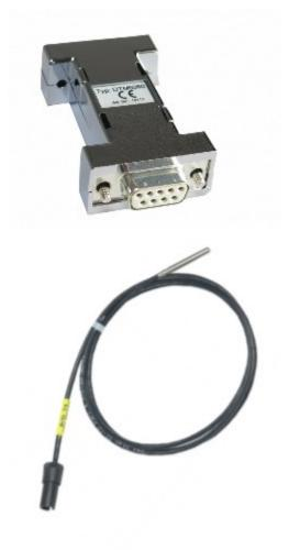
Cost-effective digital temperature logging module for the RS232 and USB interface for sensing devices with temperature resistance sensors
