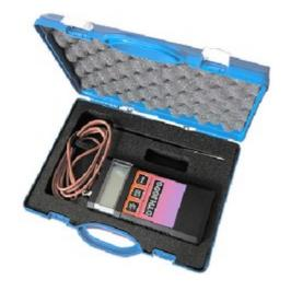
Cost-effective high-accuracy manual thermometer with a resolution of 0.01°C, controlled by a microcontroller
